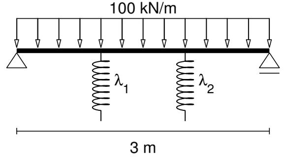
Figure 8: A beam bedded on two springs.
