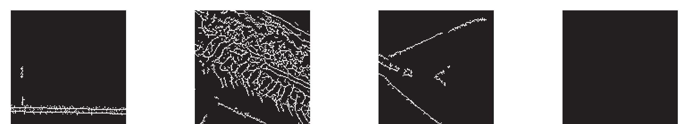
Approach by Canny-Decic filtering with high thresholds s_l = 28 and s_h = 30 .
